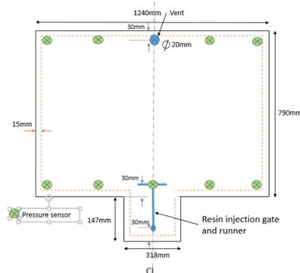
**Figure 1:** Schematic of the Panel Geometry and Sensing Equipment
