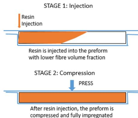
**Figure 2:** Injection and Compression Stages in the Manufacture Process
