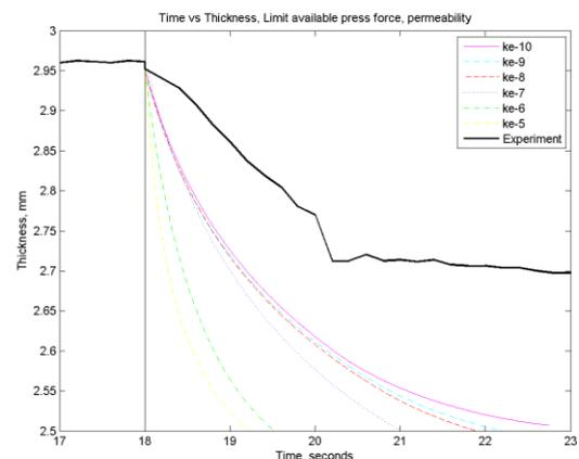
**Figure 4:** LIMS Simulation Output and Experimental Data: Top to Bottom Tool Thickness During Compression
