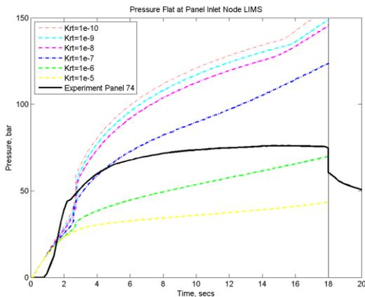
**Figure 3:** LIMS Simulation Output and Experimental Data: Pressure During Injection
